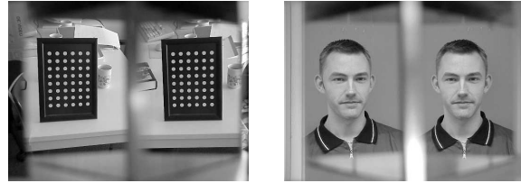
Figure 5: Stereo views in a single image, calibration plate and actual scene
