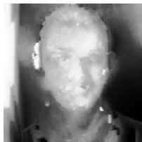
Figure 7: The disparity field, denoting for each pixel in the right image what is the displacement to the corresponding pixel in the left image
